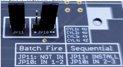
Jumper for fuel pump control (Remove the STSIGN fuse!):
